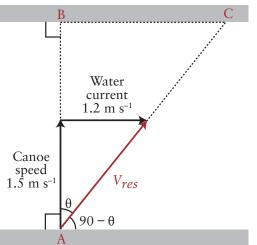
The direction in which the canoe moves makes an angle  $\theta$  with the line AB, which is perpendicular to the bank. So tan  $\theta$  = opp ÷ adj = 1.2 ÷ 1.5 = 0.8 giving  $\theta$  = 38.7°.
